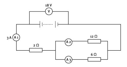
12.1 Calculate the equivalent resistance of the whole circuit. (5) 12.2 If the reading on  $A_3$  is 2 A, what is the reading on  $A_2$ ? (2) [7]
