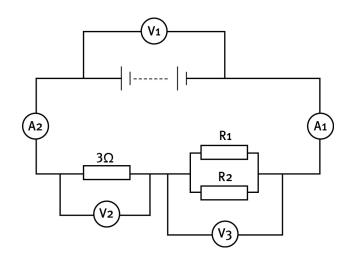
11.1 Define potential difference. (2) 11.2 What is the reading on  $V_2$ ? (2) What is the reading on  $A_2$ ? (2) 11.3 11.4 You are given that the single-series resistor has a resistance of 3  $\Omega$ . Explain why the effective resistance of the parallel pair of resistors is 1  $\Omega$ . (4) 11.5 What is the resistance of  $R_1$ ? (2) 11.6 Calculate the charge that passes through the 3  $\Omega$  resistor in 2 minutes. (4) [16]
