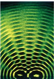
Two beads are attached to the vibrator of a ripple tank and are positioned so that they dip into the water, as shown in the photo above. The resultant pattern is shown in the second photograph.
