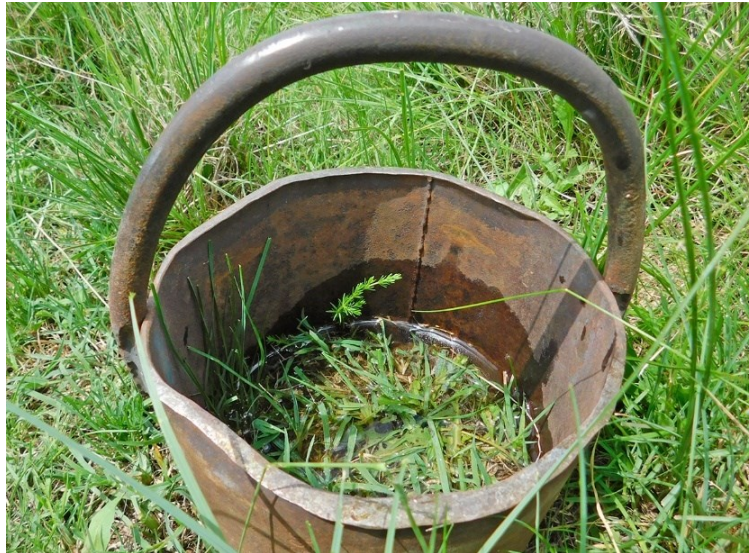
Figure 13: Water infiltration was measured by driving a 150 mm cylinder into the ground. 440 mm of water (simulating approximately 25 mm of rainfall) was then poured into the cylinder. The time taken for all water to infiltrate into the soil was then recorded.
